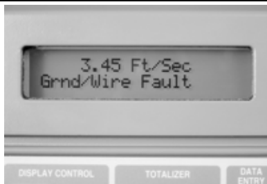
Grounding and wiring fault displays on LOI.
